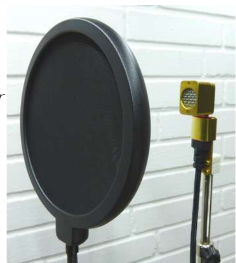
Pop-filter/Pop-shield. Diameter of the screen is 15 cm, and placed about 20 cm form the LCA1
